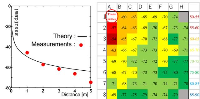
Fig. 1 Relations of the measured RSSI values to the distances ((a) one dimension (left side), (b) two dimension (right side)).
